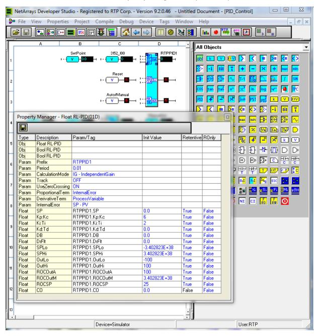
To connect inputs to outputs, you should left click on the input of one of the objects and drag it
