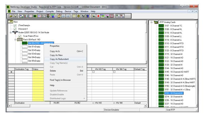
Right Click on Rack 01 / Slot01=Empty position and paste the redundant card.
