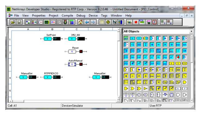
In the Object Module, grab a Float Gate Object and drop it in the cell C4.
