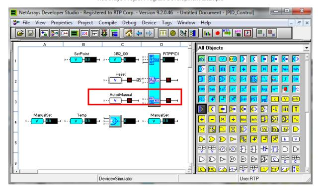
Connect the inputs to the outputs of the objects as shown in the following figure
