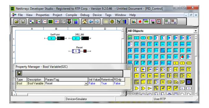
• On cell C3 in the "IP\_Control" Form, add one more Bool Variable object by repeating the above steps. Rename this new Bool Variable to Auto/Manual and set the Init Value to False.
