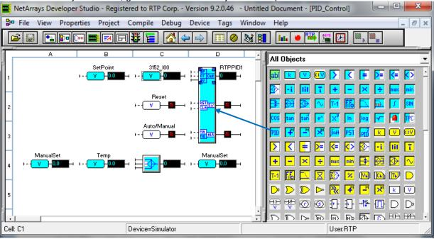
Right Click on the PID Object and select properties in the pop-up menu. Update the PID's parameters as shown in the figure below.
