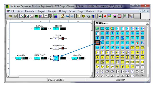
In the Object Module, grab a Float RL-PID Object and drop it in the cell D1.
