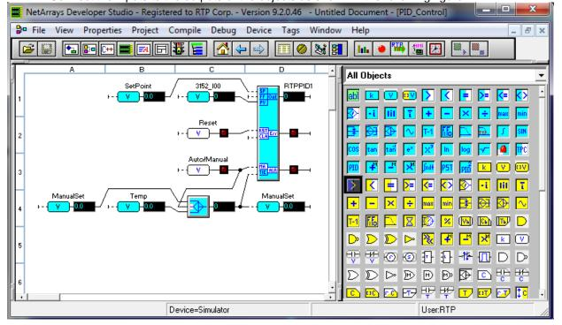
The output of the PID object will connect to the channel 0 of the 3144 Analog Output Card and add to the logic of the PID tieback.
