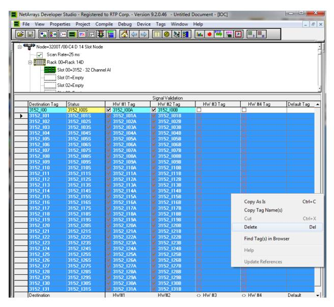
Go to the Column type of the Signal Validation display and select the option 4-3-2-1-0/V/A. This signal validation algorithm will vote the 2 input signals and output the mean of the valid inputs. In the case that none of the inputs is valid, it will output the value of the Tag located in the column "Default Tag".
