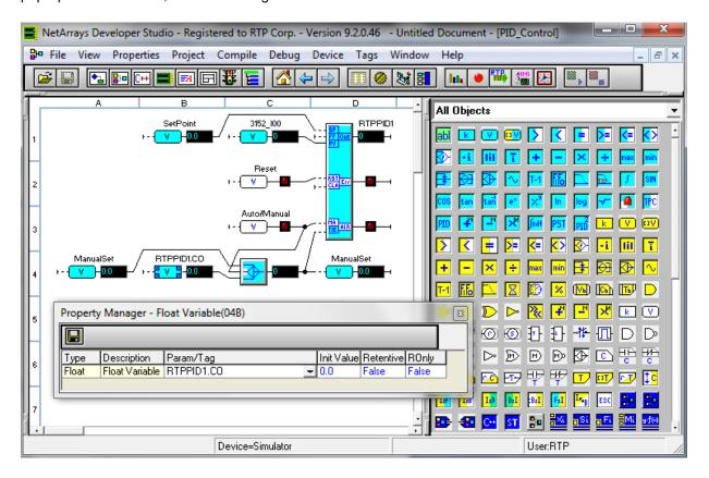
Go to the I/O configuration and right click on the card 3144 located on Rack 00/slot1. Then, select properties on the pop-up menu. In the I/O tag column of the Property Manager window, rename the tag of the channel 0 "3144O00A" with the name RTPPID1.CO. This will link the output of the PID with the 3144 card.
